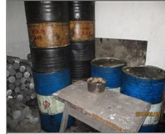
Photo of non-conformity 7.7 Lubricating oil without leakage protective device and MSDS.JPG
